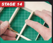
Many parts are made to measure; here I am marking the length of a cap strip by lightly scoring the wood with a scalpel, and then removing to my cutting board to cut to size. Don't attempt to cut the piece in situ, and if in any doubt about your ability to cut accurately to size then cut oversize and sand the part down; an emery board is ideal for this.
