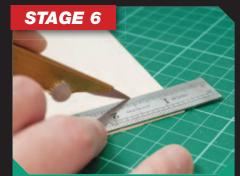
Plan on using three or four scalpel blades for a typical 'sport' size model: changing the blade as soon as it starts to drag. When cutting, try to keep the blade at 90 degrees to the wood, especially important with thicker pieces, and make several modest strokes. If having difficulty freehand cutting around curves, then cut them slightly oversize and sand down to the final shape.
