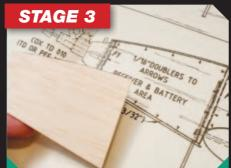
Many plans will carry indicators to aid interpretation. Here arrows are used to mark the outlines of doublers which reinforce the fuselage sides. Other signs to look out for are the centre of gravity (a circle with black quarters, or large arrow marked 'CG') and dotted lines indicating parts concealed behind
