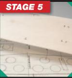
It isn't always necessary to mark out whole parts. This tailplane is largely straight lines, which will be cut with a rule, so it is only necessary to mark out the corners, and the centre line for future reference. Needless to say any curves which need to be cut freehand need to be drawn out in full.
