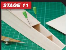
Top and bottom sheeting completes the fuselage box. Note how the grain runs across the width; although it takes longer to sheet this way the grain at ninety degrees to the fuselage sides adds greatly to the strength. Note also how the parts have been only roughly cut to size; they will be sanded down
