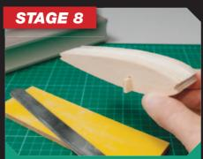
Any parts which are required to be the same, such as wing ribs or sheet fuselage sides, should be sandwiched together and lightly sanded to ensure that all the pieces are exactly the same size and shape. The more accurate we can make our parts the easier assembly will be, and the better the fit of parts, the stronger our airframe will be. It is better to have parts which are a tight fit, and relieve them with emery board, that to have gaps which will weaken our structure considerably.
