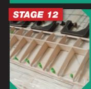
The wings are built over the plan, after first covering with cling film. Semi symmetrical sections can be built flat, but symmetrical sections such as this one require a support piece to be placed at the rear. It is important that whatever you use as your building board is completely flat, and able to accept pins. I usually use a piece of plasterboard fixed onto a kitchen worktop. After every couple of projects or so the board is removed and replaced.
