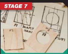
Note the markings on the plan for these formers. The wavy line on F1 denotes that this is to be made of plywood, and the straight lines on F3 denote the grain direction for the balsa. For simple geometric shapes like these it is better to simply measure them and draw them into the wood using a rule and square rather than tracing.
