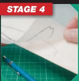
Construction begins by producing a kit of parts, and to do this we need to transfer the shapes from plan to wood. There are many methods for doing this; some make photocopies and, using a hot iron, transfer the dye to the wood. An alternative is to cut out the copies and 'tack glue' them onto the wood. Others simply prick the shapes through with a pin, or trace through the plan onto the wood, leaving an indentation. Here I use good old fashioned tracing paper.
