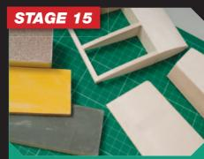
Thorough and accurate sanding is a vital part of any build. Always use some form of sanding block; I use Perma-Grit tools for the rougher grades, and glue sandpaper to MDF blocks for the smoother stages. Start off rough and then work down to smoother grades (Remember to do this in a well-ventilated area and wear a mask). Run your finger along any joints to ensure that they are smooth.
