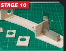
Fuselage assembly is sometimes done over the plan or, as is the case here, by attaching the two main formers in the parallel area of the fuselage. Care needs to be taken that these are square to the fuselage side and in the correct position as denoted by the plan. When these are dry the second side is placed on top, using squares all around to ensure that it is exactly atop the first.
