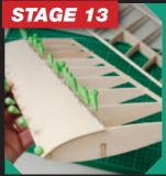
Most wings employ sheeting forward of the main spar to form a 'D' box. It is important that plenty of pins are used to ensure that the wood adheres well to the curve of the rib profile. For sharper bends it may be necessary to soak the wood in water to easier obtain a curve. As with the fuselage sheeting, note how the wood has been cut oversize, to be sanded to an accurate profile later.
