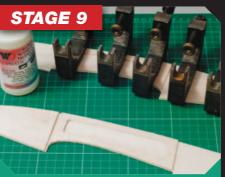
On this build I started with the fuselage, and this starts by attaching the doublers to the fuselage sides. Use a slow setting glue for this such as epoxy, aliphatic or PVA, as these give more time to accurately position parts. After positioning the pieces, use heavy weights or clamps to ensure good adhesion. Be sure to prepare one left and one right hand panel !!
